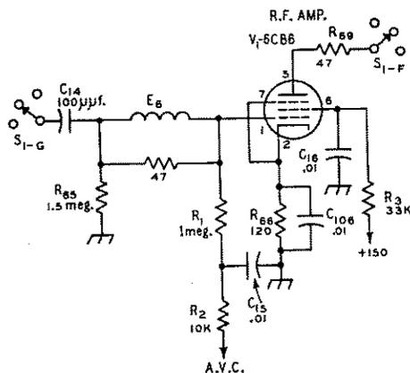
Fig. 1 — Revised 75A-2 r.f. stage circuit when replacing 6AK5 with 6CB6. All resistors  $\pm 10$  per cent values,  $\frac{1}{2}$  watt. See Appendix I.
