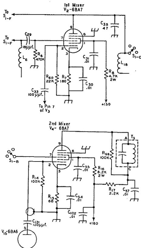
Fig. 4 — Revised mixer circuits for the 75A-2 where replacing 6BE6s with 6BA7s. All resistors = 10 per cent values, ½ watt, unless otherwise noted. See Appendix III.
