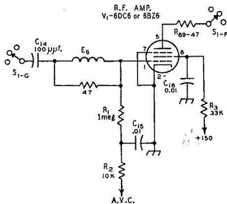
Fig. 2 — Revised r.f. stage for use of low cross-modulation 6DC6. All resistors  $\pm 10$  per cent values,  $\frac{1}{2}$  watt. See Appendix II.
