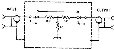
Fig. 3 — R.f. attenuator of 21-db. loss for reducing signals at antenna terminals. All resistors = 10 per cent values, ½ watt.
