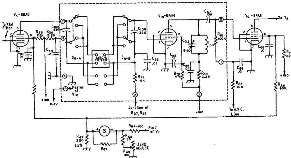
Fig. 5 — Circuit modifications for using 455B mechanical filter. All resistors  $\pm 10$  per cent values,  $\frac{1}{2}$  watt.  $R_{87}$  — 150 ohms. If 455C mechanical filter is used, the following values change:
